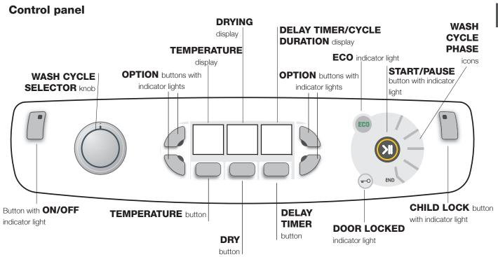
Button with **ON/OFF** indicator light: press this briefly to switch the machine on or off. The green indicator light indicates that the machine is switched on. To switch off the washer dryer during the wash cycle, press and hold the button for approximately 3 seconds; if the button is pressed briefly or accidentally the machine will not switch off. If the machine is switched off during a wash cycle, this wash cycle will be cancelled.
